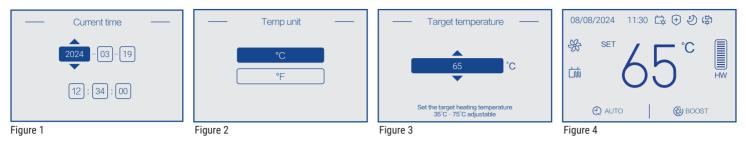
When the device is powered on for the first time, the screen lights up and enters startup mode. Begin setup by selecting the initial settings. Adjust the current time, set the temperature unit (°C/°F), and set the target temperature by turning the rotary dial. Press the rotary dial to confirm each selection. Set the temperature to 60°C (AUTO - Standard Recovery mode is set by default).
